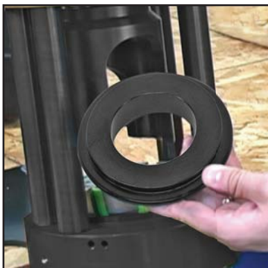
Install the pusher plate on top of the die set. Note the "This Side Up" notation.
