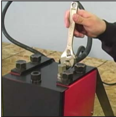
Disconnect and discard the existing T400 head unit. It is recommended that the hose be replaced with a new 4300 psi working
