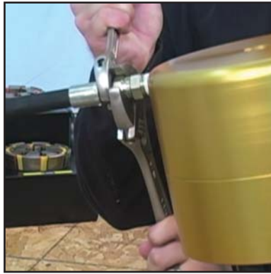
Connect the T400 Power unit to the new Continental Products crimp head. Do not readjust the hydraulic unit to exceed 4300 psi.
