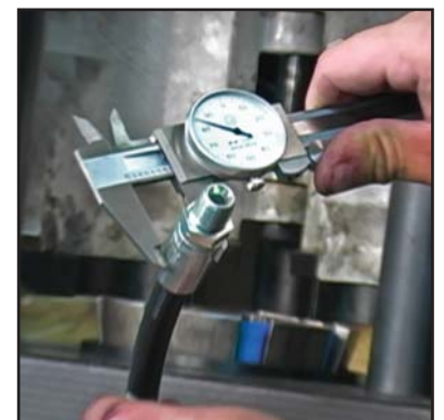
Release the hydraulic pressure and withdraw the hose. Always measure the completed fitting.
