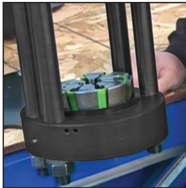
Select the correct flex cage die from the chart and insert it in the cone base.
