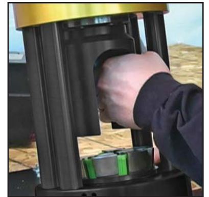
Install the pusher on the stud on the bottom of the hydraulic ram
