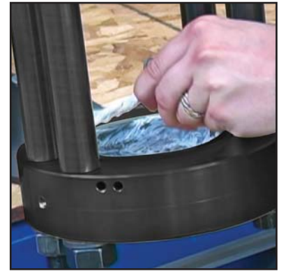
Lubricate the cone base with the grease furnished with the kit.
