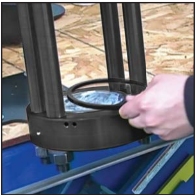
Select the correct spacer ring and place it on top of the cone base. A zero indicates no holes, 1 indicates 1 hole etc.
